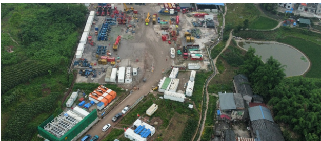
The energy storage system + gas power generation is applied in a block in Chongqing to power the fracturing platform
